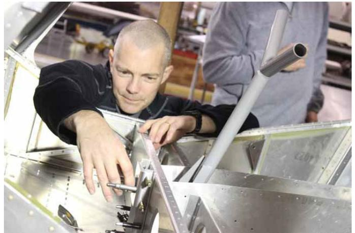
Matt has been working in the cabin area on the control stick torque tube.
